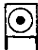
BORESIGHTING AND ZEROING TARGET FOR THE MAIN GUN, USED TO BORESIGHT COAXIAL MACHINEGUN.
